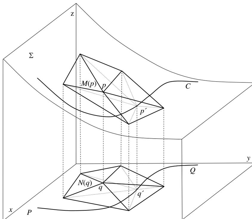
Figure 1: The relocation of node  $p \in \Sigma$  is performed in the plane  $P$  by projecting  $q$  on  $Q$  and, consequently,  $p$  on  $C$ .
