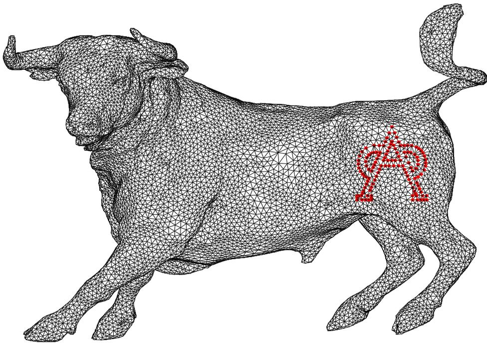
Figure 6: Mesh of a bull with an emblem inserted in its back.
