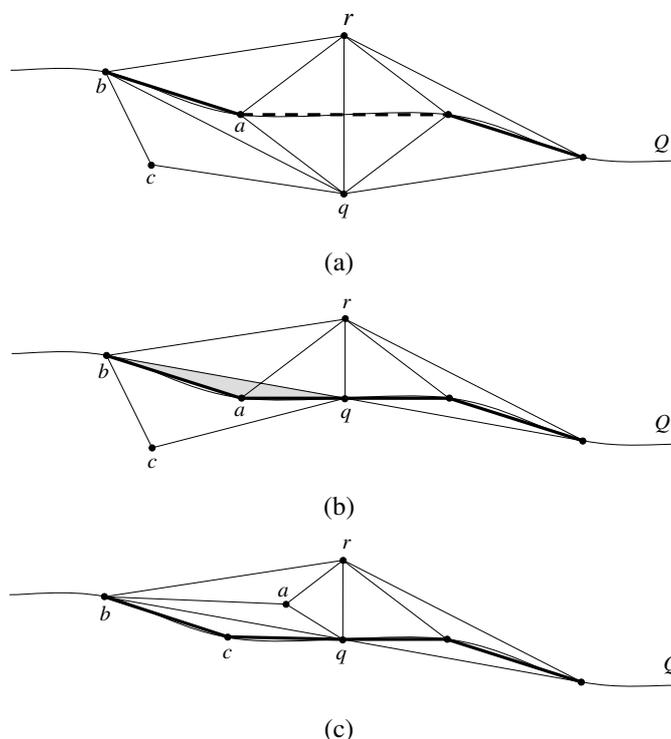
Figure 4: The dashed line is non-recoverable without tangling the mesh (a). The free node  $q$  is enforced to be projected (b). The tangled triangle  $abq$  is untangled and the node  $c$  is also projected (c).
