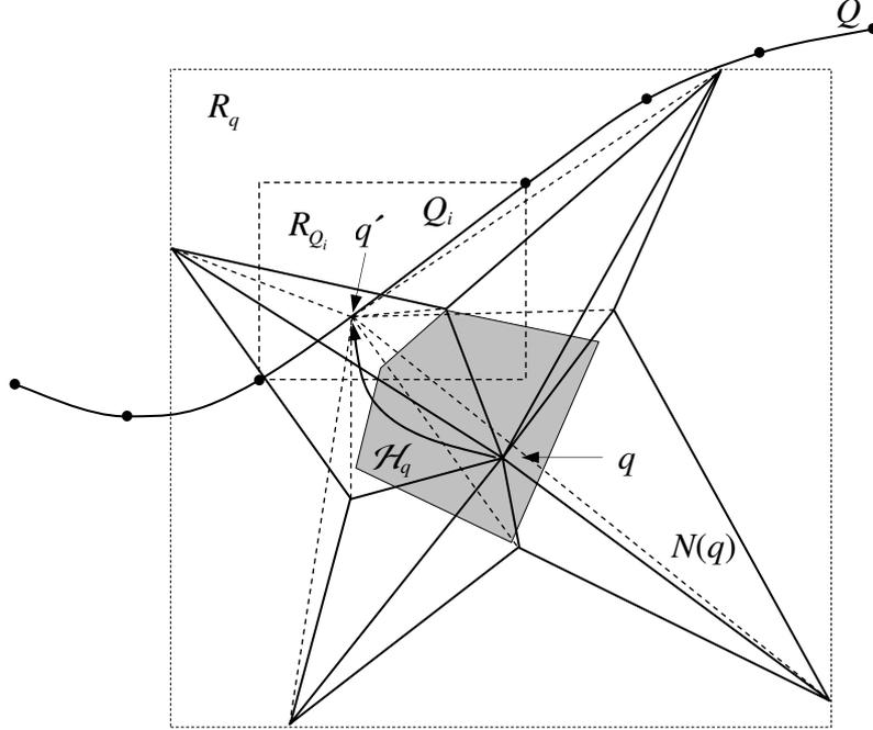
Figure 3: The figure shows the situation in which  $R_q \cap R_{Q_i} \neq \emptyset$ , but node  $q$  is not projectable because the optimal position for the free node,  $q'$ , is outside the feasible region.
