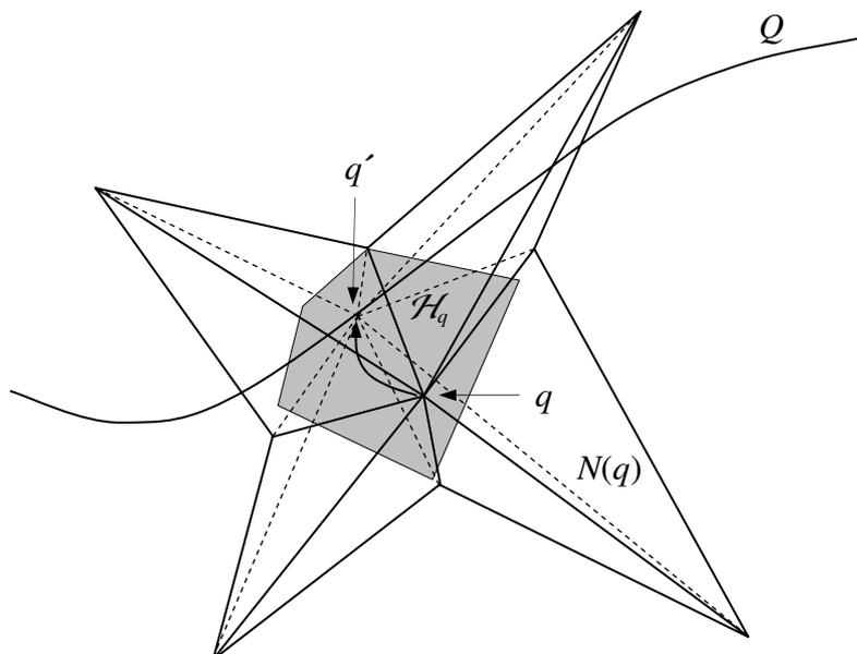
Figure 2: The curve  $Q$  intersects the feasible region  $\mathcal{H}_q$  (in gray) and, therefore, the node  $q$  is projectable, being  $q'$  its optimal position on the curve.
