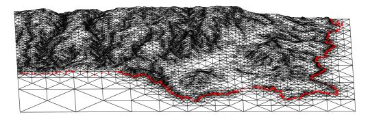
Figure 3: Region defined in the north west of Gran Canaria Island. Contour plots and initial mesh to be adapted.
