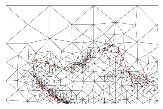
Figure 6: A detail of the coast in the north west of Gran Canaria Island corresponding to the adapted mesh.
