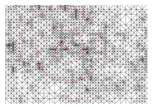
Figure 7: Region defined in the surrounding of Arucas Mountain (Gran Canaria Island). Contour is defined as an spiral line around the mountain to which the initial mesh must be adapted.
