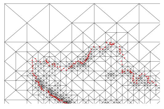
Figure 5: A detail of the coast in the north west of Gran Canaria Island corresponding to the not adapted mesh.
