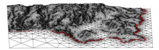
Figure 4: Region defined in the north west of Gran Canaria Island. Contour plots and adapted mesh.
