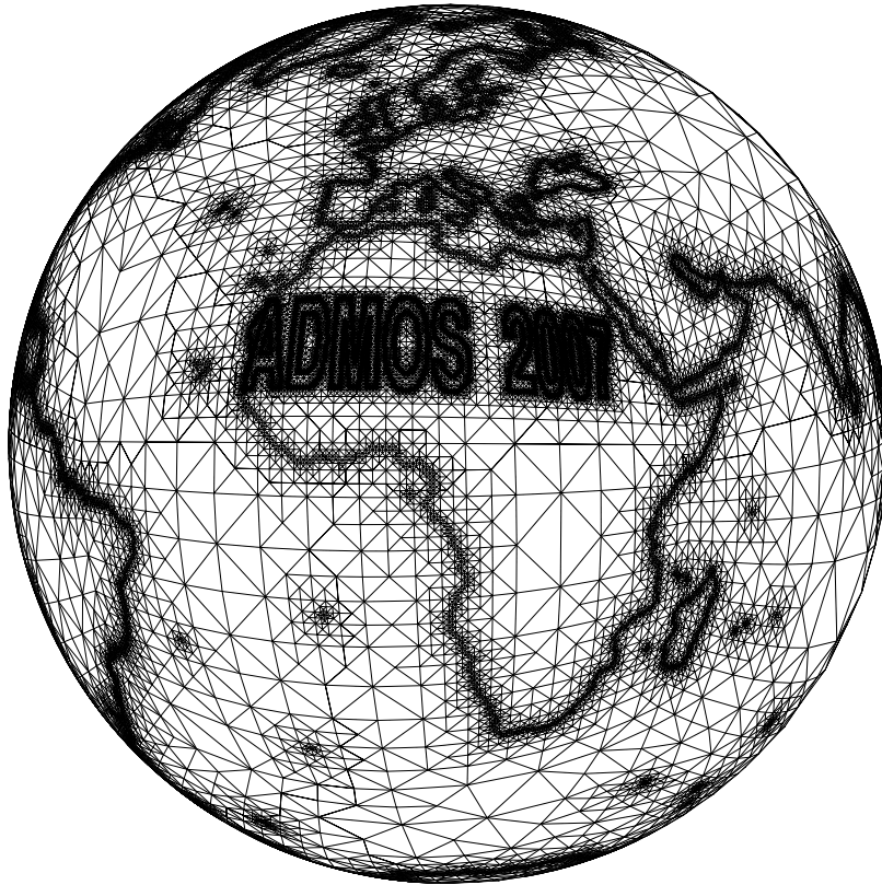
Figure 1: Resulting adaptive tetrahedral mesh of the Earth after applying the refinement/derefinement procedure on the meccano (one cube) and radial node projection from meccano faces to Earth surface
