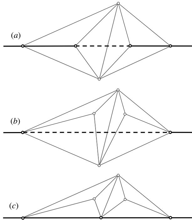
Figure 2: The line (in bold) is non-recoverable if the two extreme nodes are not moved (a). The extreme nodes are removed from the line (b) until another one takes its place (c)
