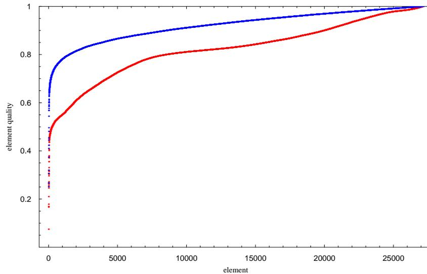
Figure 15: Quality curves for the initial (dashed line) and optimized (solid line) meshes for the screwdriver.
