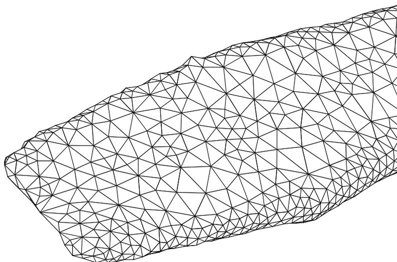
Figure 14: Detail of the optimized mesh of the screwdriver after four iterations.
