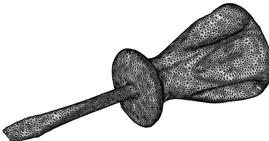
Figure 12: Optimized mesh of the screwdriver after four iterations.
