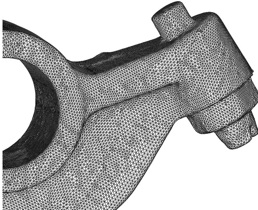
Figure 4: Detail of the optimized mesh
