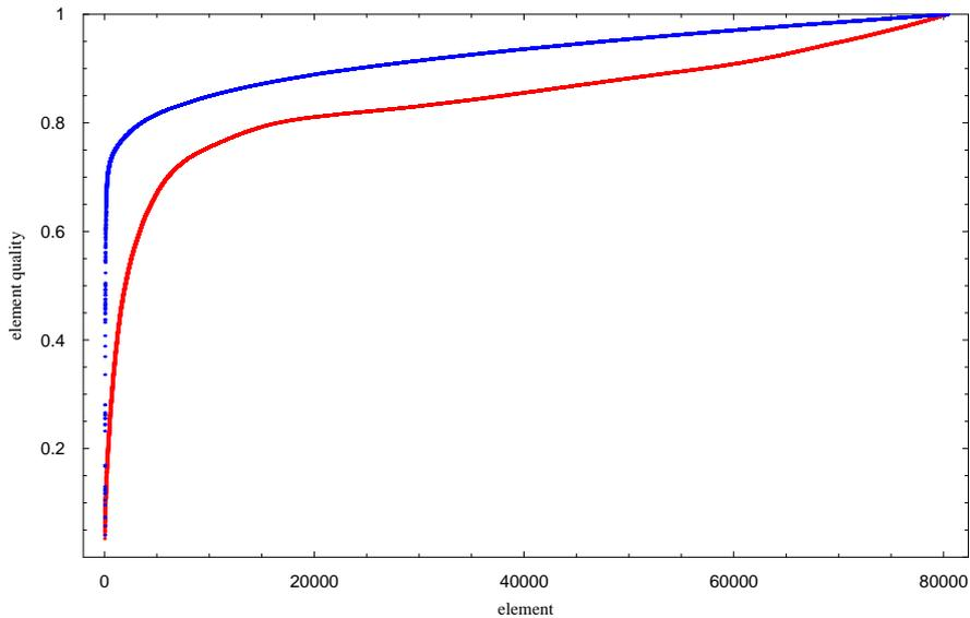
Figure 5: Quality curves for the initial and optimized meshes
