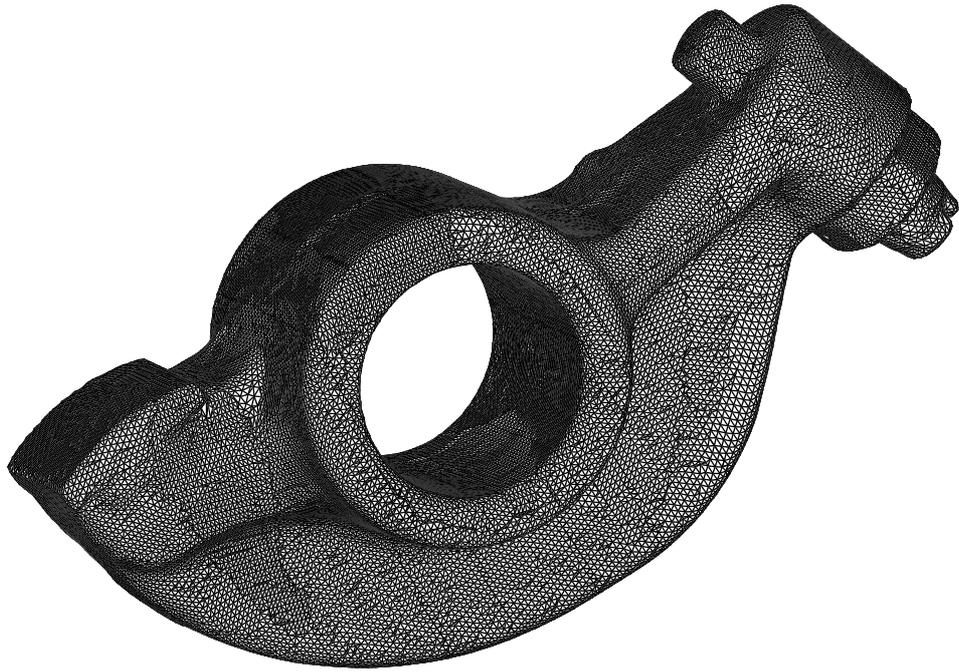
Figure 2: Original mesh of the rocker arm
