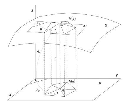
Figura 1. Local surface mesh and its associated parametric mesh.
