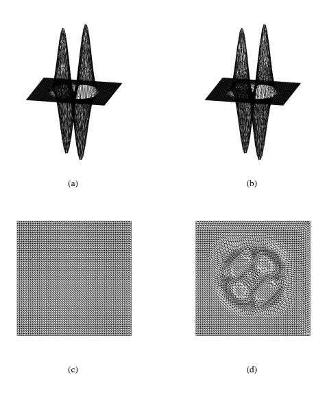
Figura 5. Lateral view of the initial surface mesh (a), optimized surface mesh (b), initial parametric mesh (c) and optimized parametric mesh (d)
