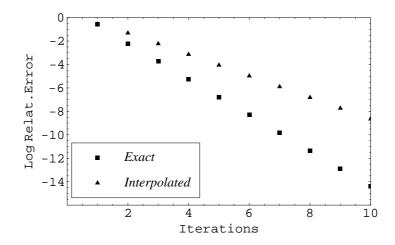
Figura 4. Convergence of the local process. Logarithm of the relative error in terms of the number of iterations.
