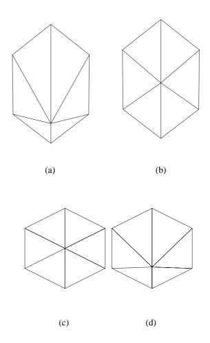
Figura 3. Frontal view of the initial surface mesh (a) and its projection on the plane (c). Frontal view of the optimized surface mesh (b) and its projection (d)
