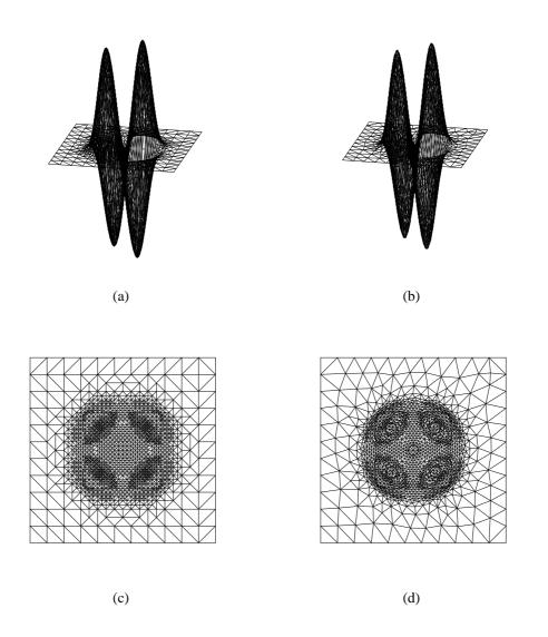
Figura 6. Initial surface mesh with refinement (a), its optimized surface mesh (b), refined parametric mesh (c) and its associated optimized parametric mesh (d)
